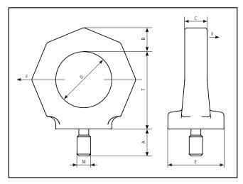
NB: Recommended for use in applications where eye bolt needs adjustment to direction of pull.
