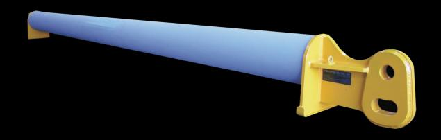
The Maxilug 80 allows users to create their own custom length, medium-lift spreader bar utilizing these heavy duty end units. Designed to accomodate readily available line pipe, Maxirig can supply the units as is or with various pipe lengths to facilitate lift spans from 2 metres up to 13 metres.
