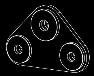
When using multiple sling legs this device provides a means of equalising forces within the legs. Connection is made via standard Grade "S" bow shackle and can be used with chain, wire rope or synthetic slings. Ideal in compensating for differences in load lift points and sling lengths.
